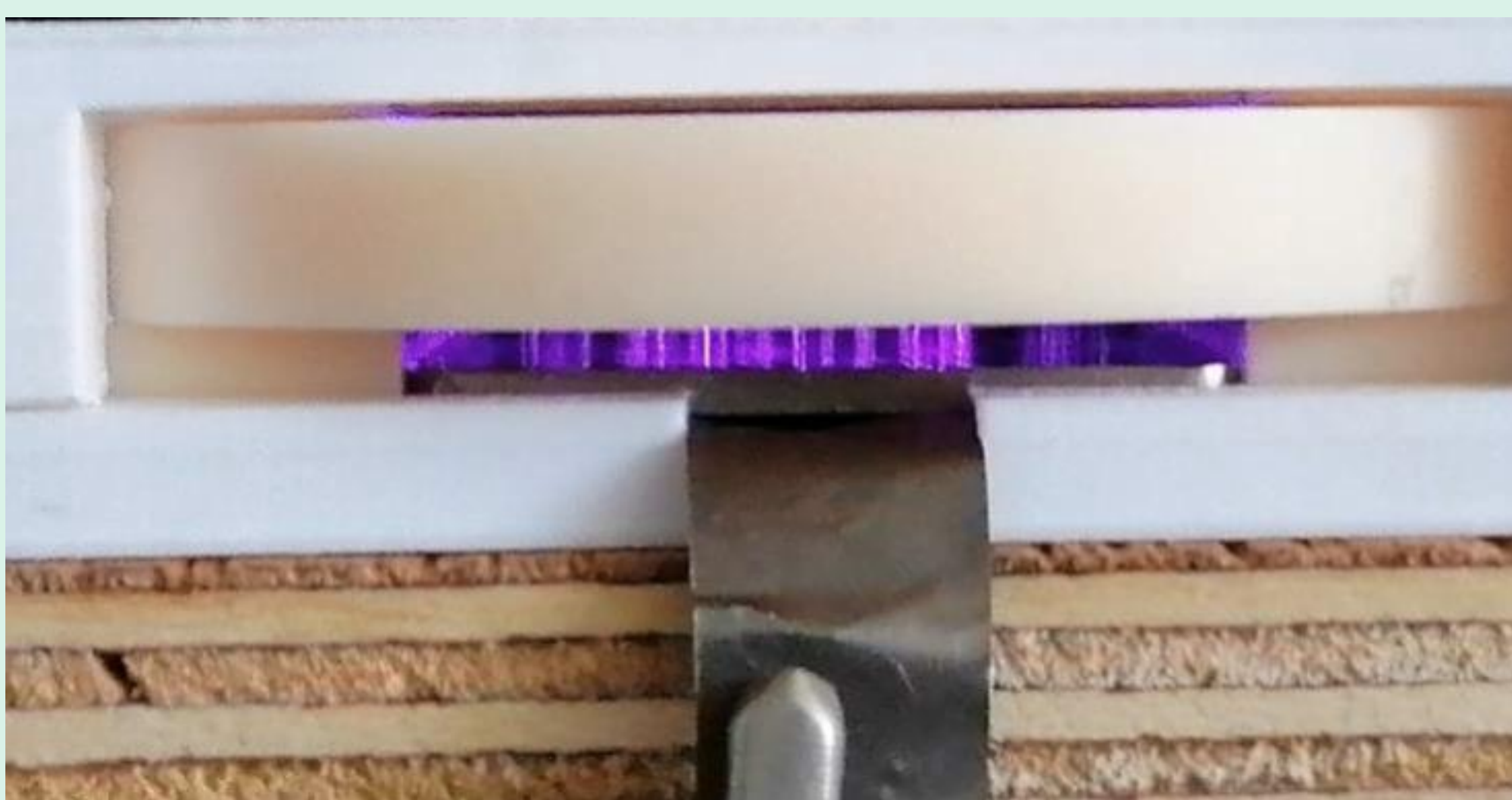
Fig. 1 : In-house atmospheric DBD-plasma reactor for the treatment of polymer foils
