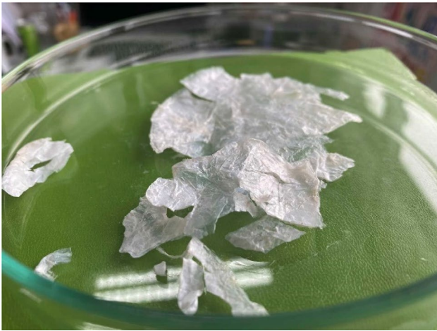
Fig. 8 Produced cellulose from PLA degradation liquid residues
