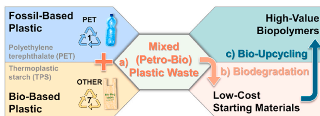
Fig. 2. Schematic detailing the main stages of the proposed biotechnological route for the end-of-life (EoL) management of mixed plastic waste: a) preparation of a model mixed (petro-bio)plastic (PET-TPS) system; b) biodegradation of mixed (petro-bio)plastics resulting in low-cost starting materials; and c) bio-upcycling of low-cost waste-derived materials into new high-value eco-polymers.
