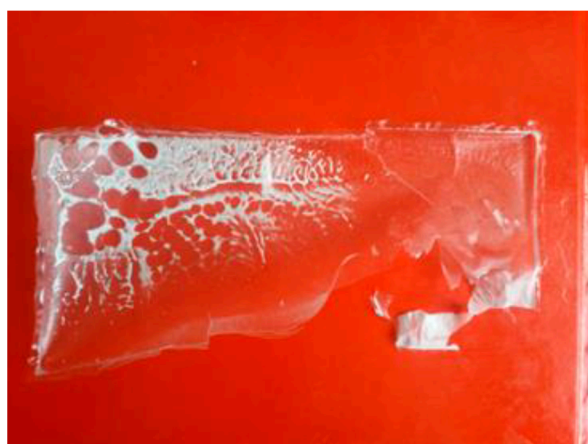
Figure A1. CA-based film with 10% of thymol obtained by the solvent casting method; unpublished data from the study Zizovic et al. [10].
